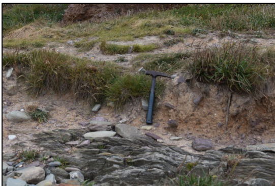
Ballycroneen Beach, cliff exposure showing coarse, rounded pebbles of raised beach deposit resting on rock platform, and overlain by matrix-supported till with very large cobbles.
