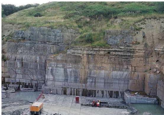
Limestone is sawn out in massive blocks for use as cladding slabs.
