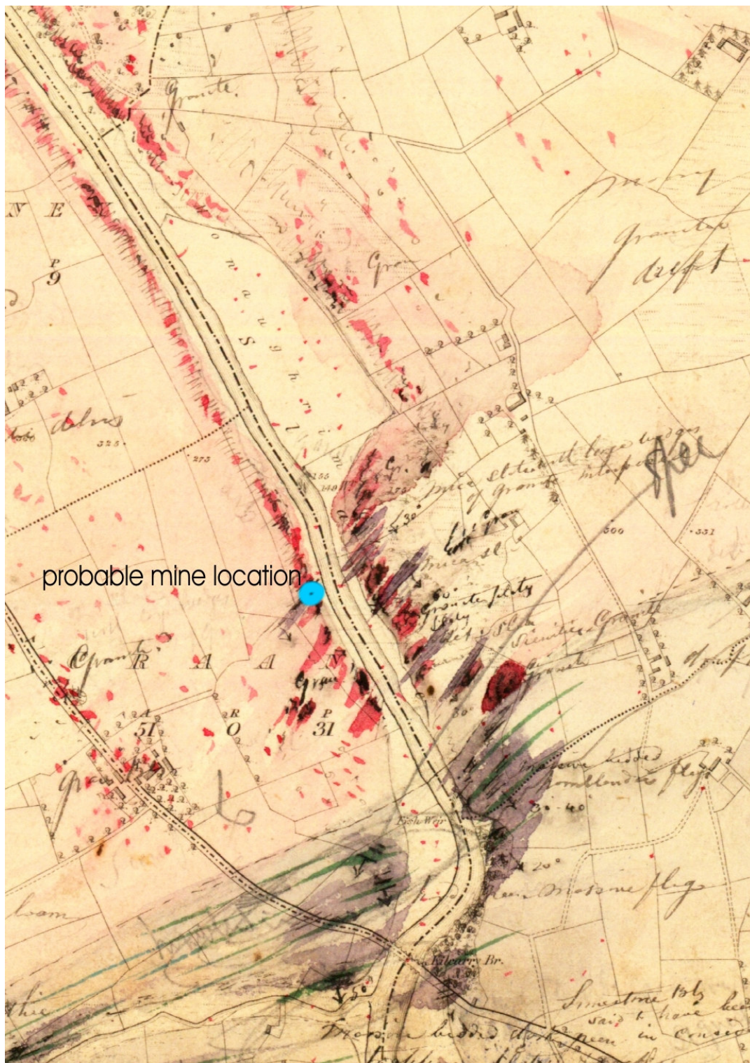
Enlarged extract of GSI 6 inch to the mile 19 th century fieldsheet, showing probable mine location within the granite outcrop (coloured pinky red), where granite and schists (coloured purple) are intermixed.
