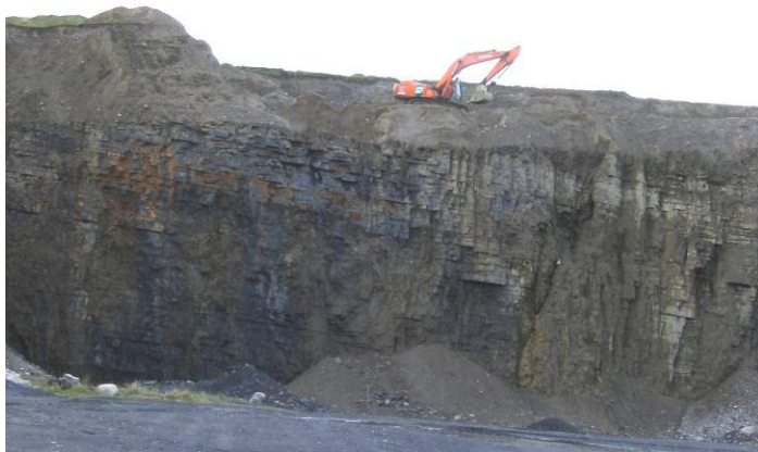
The depth of overburden is shown on this image
