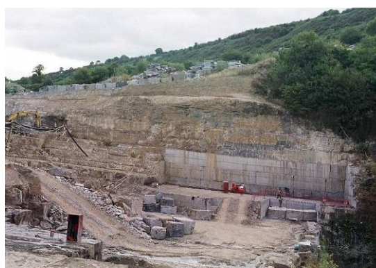
The westerly dip of the limestone beds is apparent in this view of the quarry.
