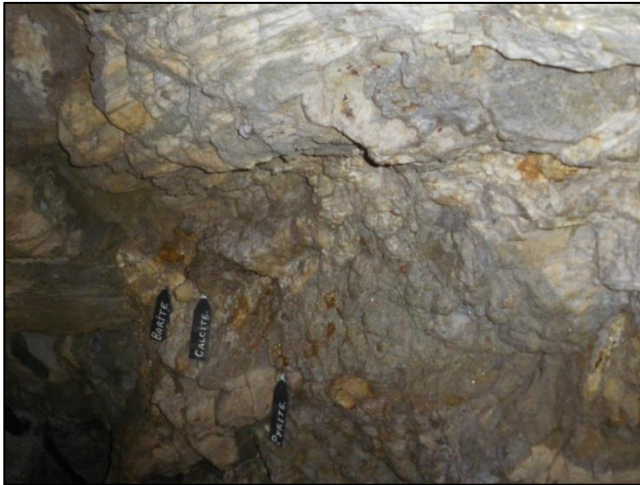
Underground: striped marbles of Lakes Marble Formation above calcite lode with barite and pyrite.
