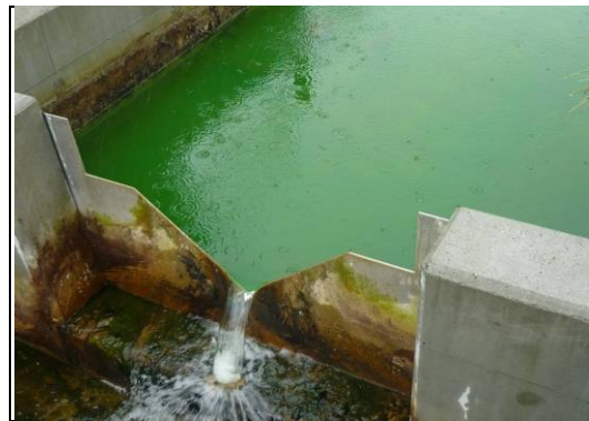
Slight greening of the spring water following dye injection at Kiltullagh Lough, July 2010.
