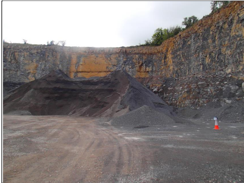
The main face in McTigue Quarry, showing bedded limestones overlying massive rock.
