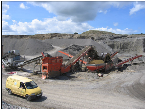
Above: Machinery used to refine the extracted gravel. Right: Exposed sand and gravel within the hill in the background. Settling pond can be seen in the foreground.
