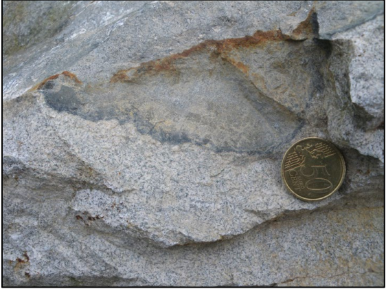
Brecciated dolerite fragments within granite vein (left). Dark, fine-grained hornfelsed zone at margin of dolerite intruded by granite (right). Granite has undulating contact surface.
