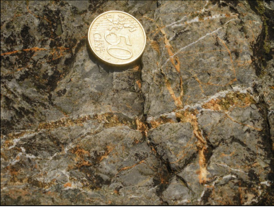
Yellow sphalerite in cross-cutting veins and fractures on foreshore (left); sphalerite and chalcopyrite in quartz veins in boulder from church wall (right).
