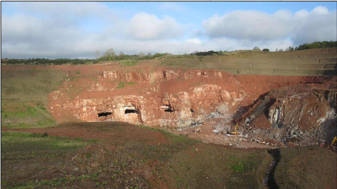
Two gypsum horizons are visible with old mine workings (pillars and stalls) intersected within the lower, thicker bed.
