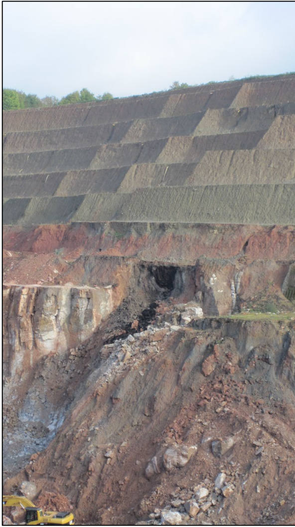
Left: Gypsum beds with a karstic doline filled with interglacial peat and a glacial till overburden in benches above. Right: Gypsum rock being broken for loading, after blasting.
