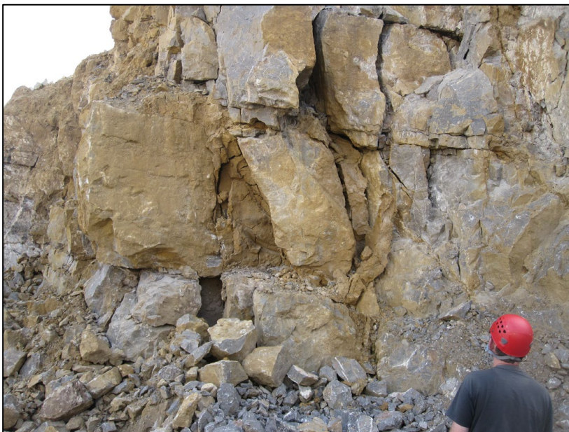
Left: A rare section of karstified limestone in the quarry, with enlarged joints and voids.
