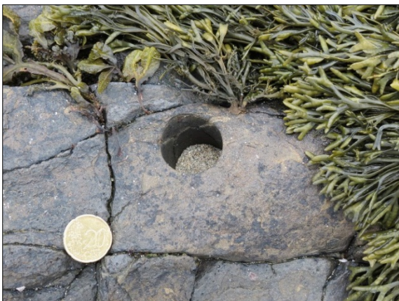
Palaeomagnetic sampling drill hole in dolerite dyke.
