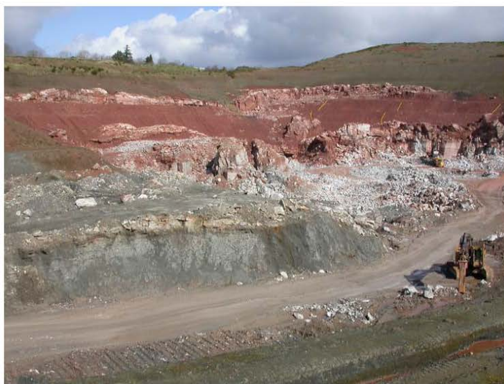
Red Permian mudstone and gypsum, and grey rotted basalt, at the Knocknacran opencast mine.
