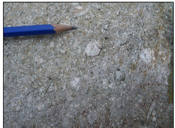
Andesite agglomerate of the Carrickatee Formation (left) and in close-up (right) showing angular clasts.
