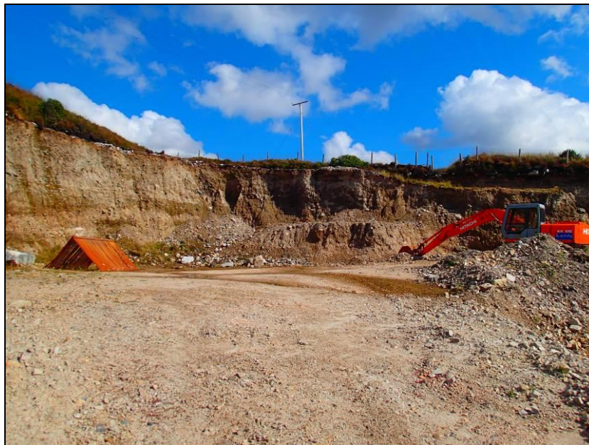
Melt out tills exposed in one of the pits in Meenanillar.
