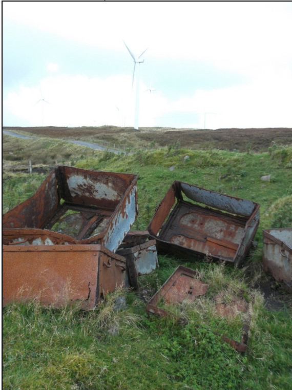
Rusting hutches for carrying coal on rails.
