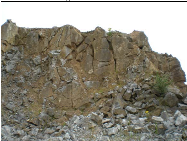
View of karstified limestone at northern face of quarry, showing epikarst – expanded joints and fractures in top few meters of limestone bedrock.
