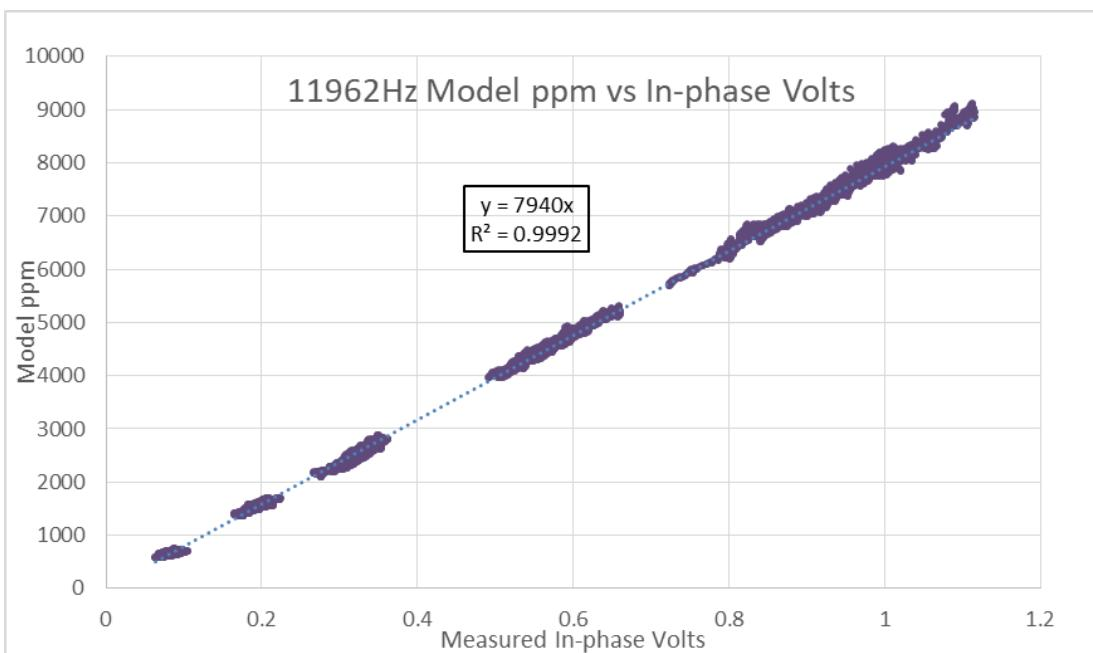
Figure 18: SGFEM 11962 Hz In Phase Seawater Calibration
