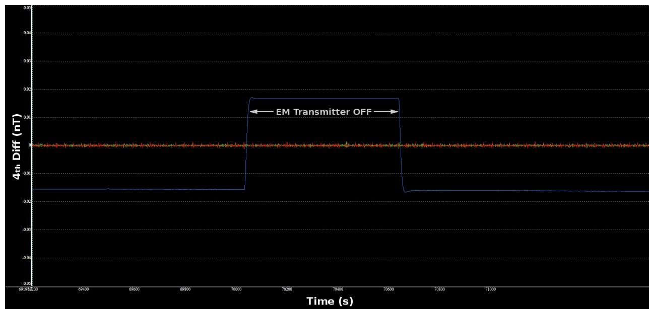
Figure 21: EM transmitter noise test, showing the 4<sup>th</sup> difference of the tail and wing magnetic sensor traces.
