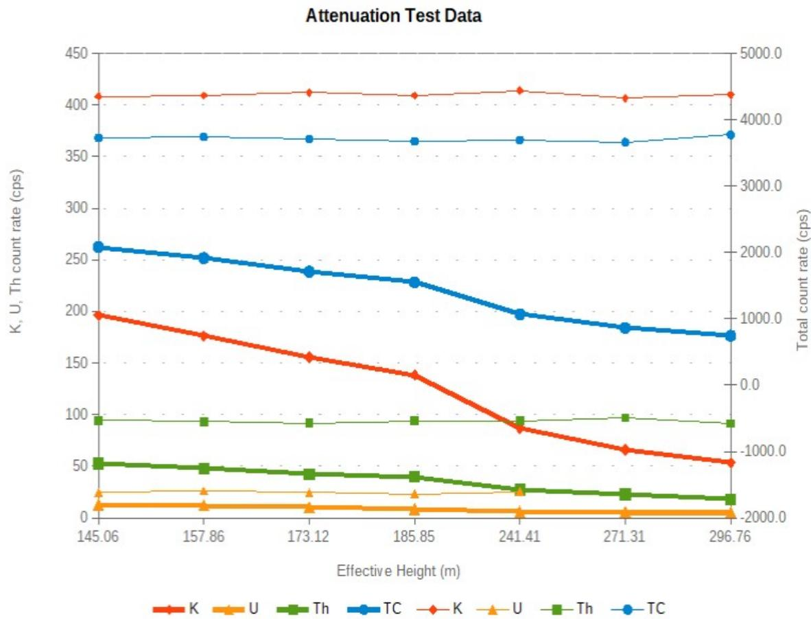
Figure 4: Spectrometer attenuation test: thick lines are recorded data, thin lines are data corrected to an effective height of 60 m using the attenuation coefficients derived.
