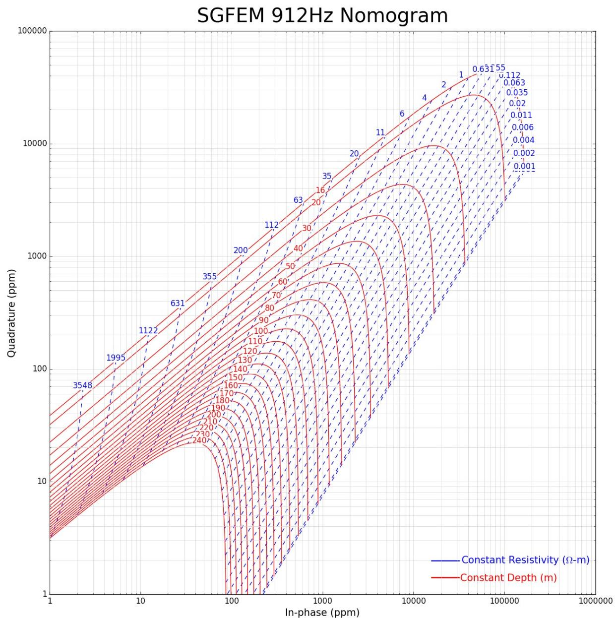
Figure 25: SGFEM 912Hz Nomogram
