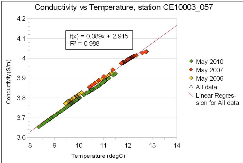
Figure 14: Conductivity variation with temperature
