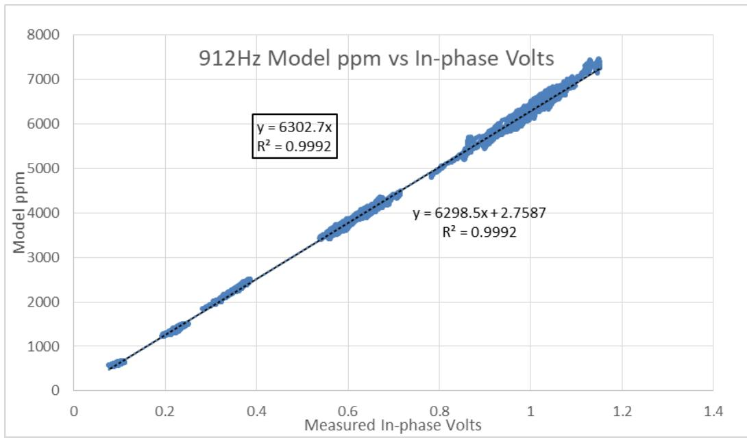
Figure 16: SGFEM 912 Hz In Phase Seawater Calibration
