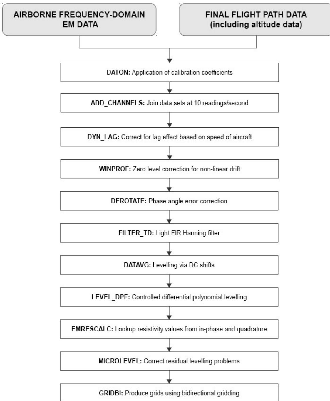
Figure 24: Frequency Domain Electromagnetic Data Processing Flowchart
