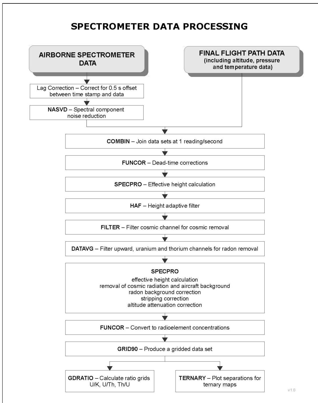
Figure 23: Spectrometer data processing flowchart
