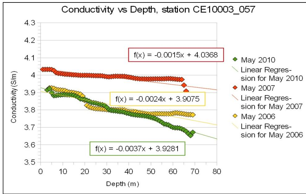
Figure 13: Conductivity variation with depth
