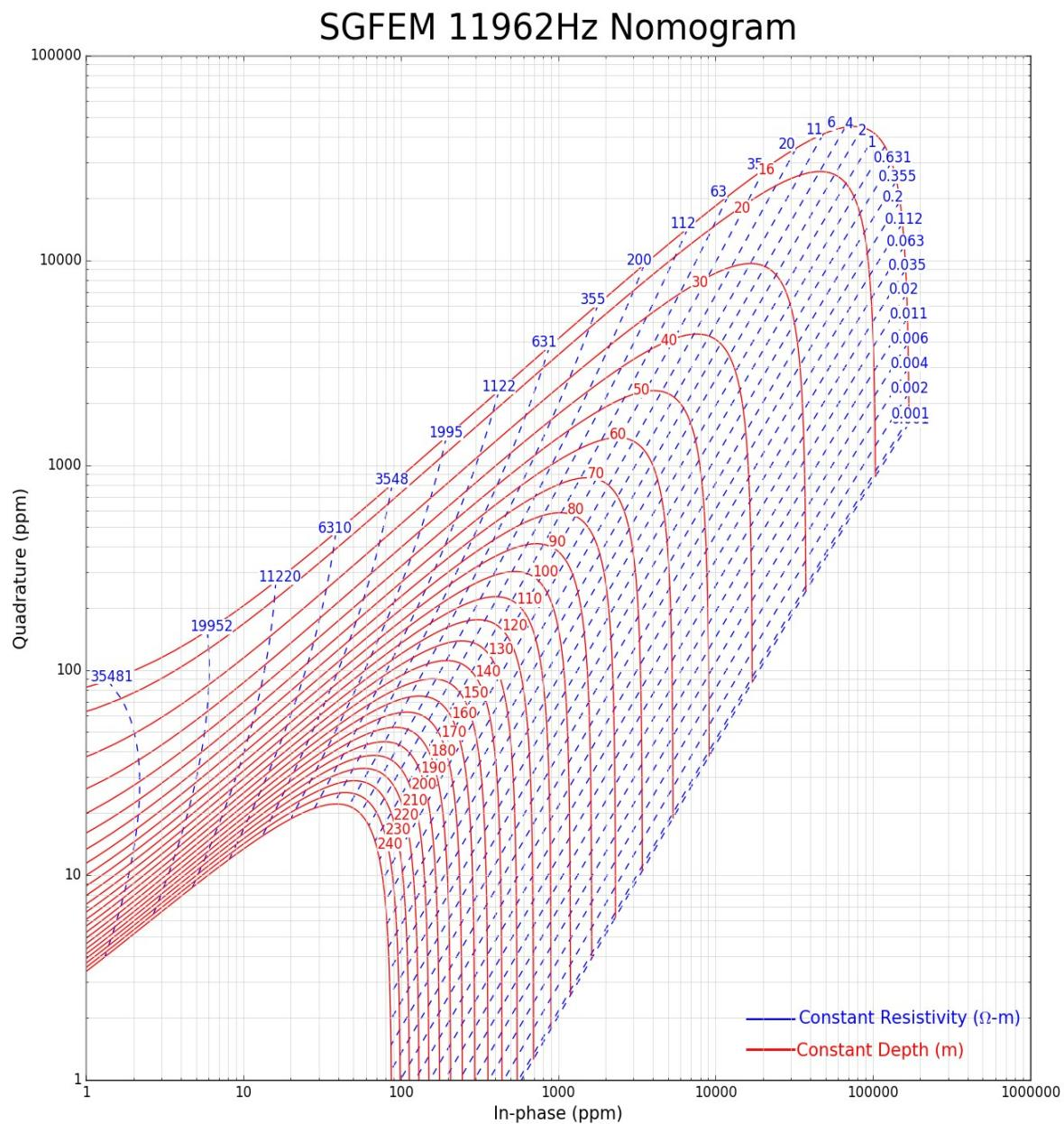
Figure 27: SGFEM 11962Hz Nomogram
