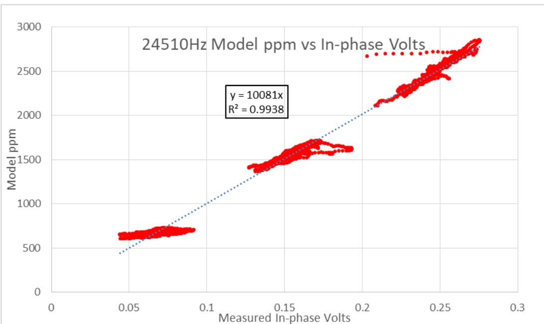
Figure 19: SGFEM 24510 Hz In Phase Seawater Calibration
