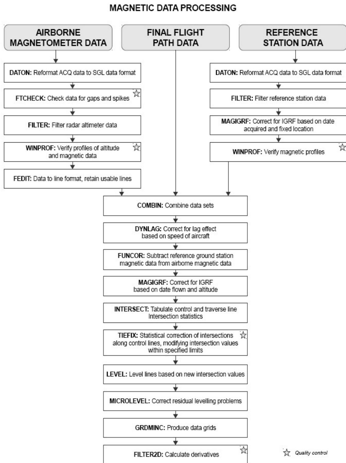
Figure 22: Magnetic data processing flow chart
