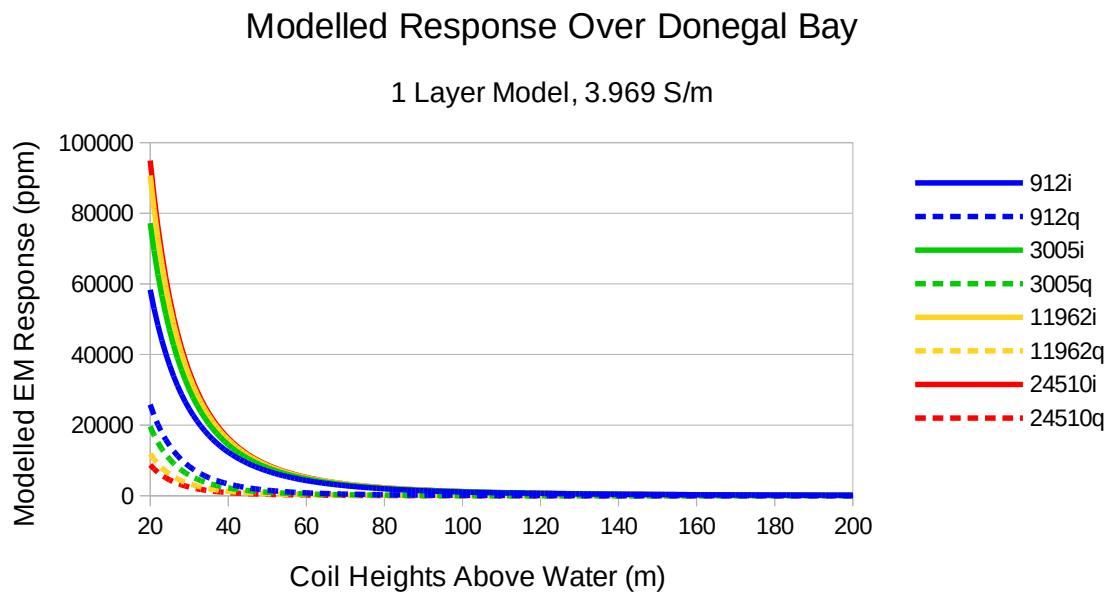
*Figure 15: Modelled EM response vs. Coil height above water over Donegal Bay*
