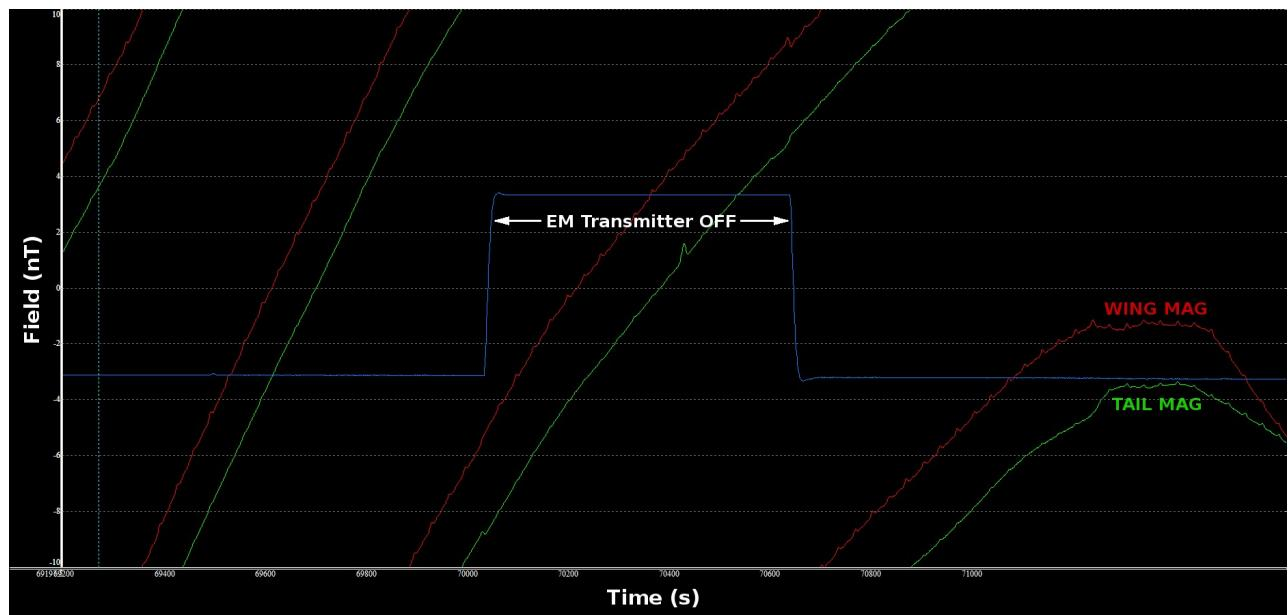
Figure 20: EM transmitter noise test, showing tail and wing magnetic sensor traces.
