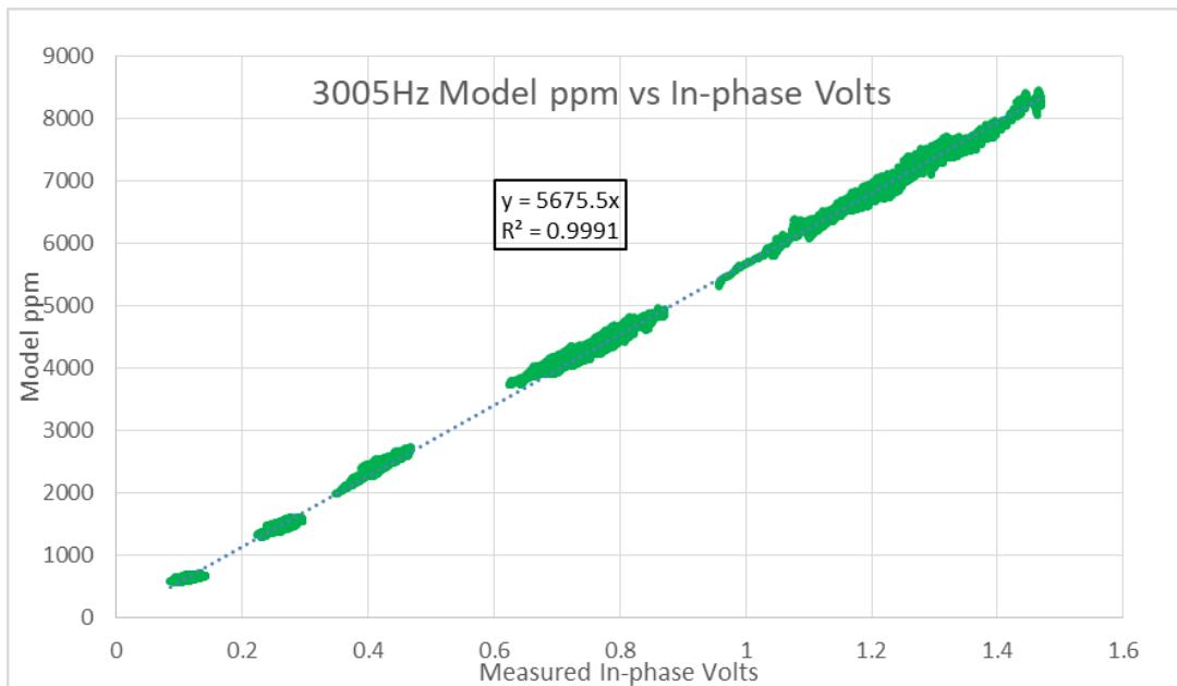
Figure 17 SGFEM 3005 Hz In Phase Seawater Calibration
