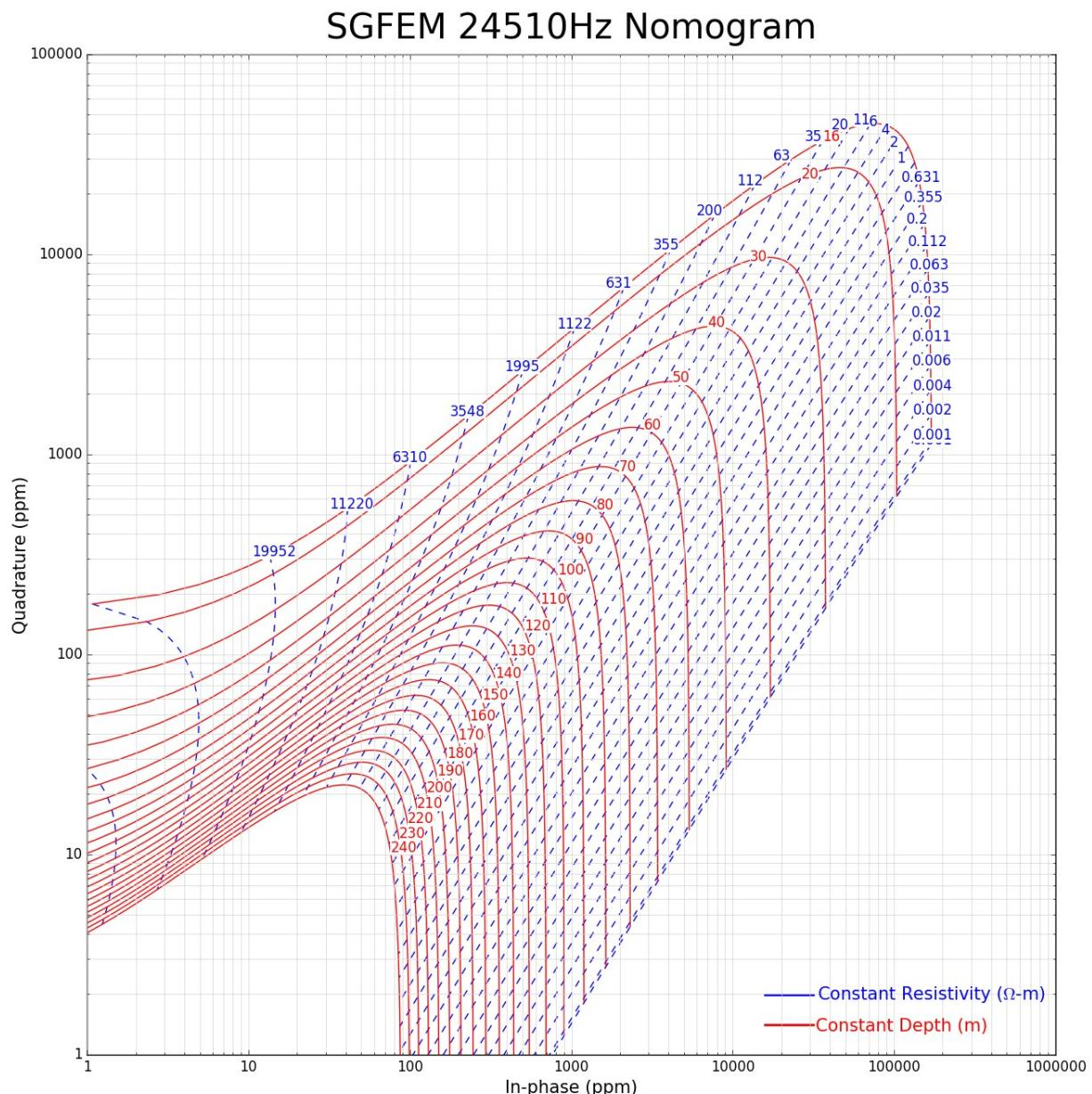
Figure 28: SGFEM 24510Hz Nomogram
