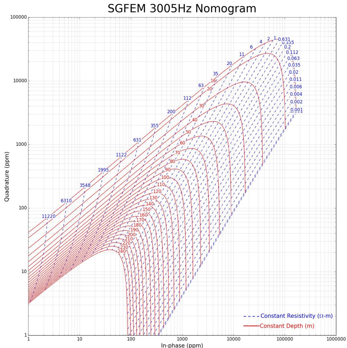
Figure 26: SGFEM 3005Hz Nomogram
