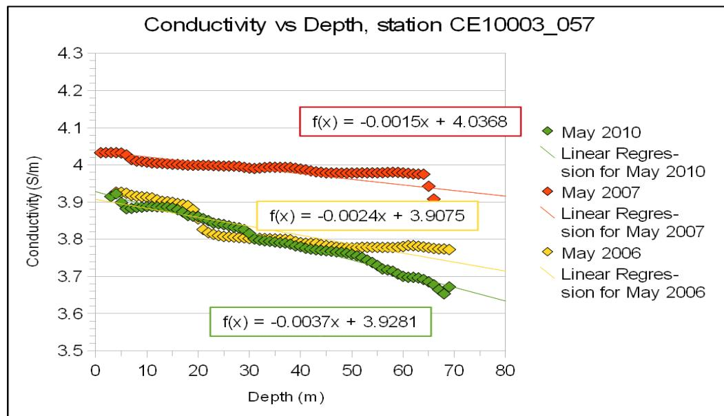
*Figure 16: Conductivity variation with depth*
