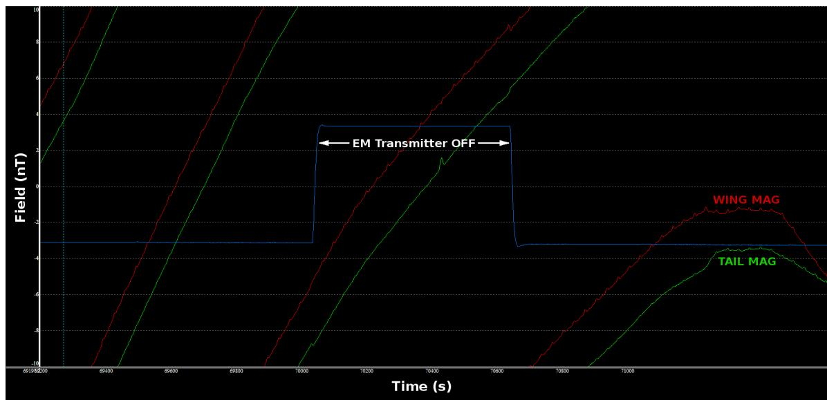
Figure 25: EM transmitter noise test, showing tail and wing magnetic sensor traces
