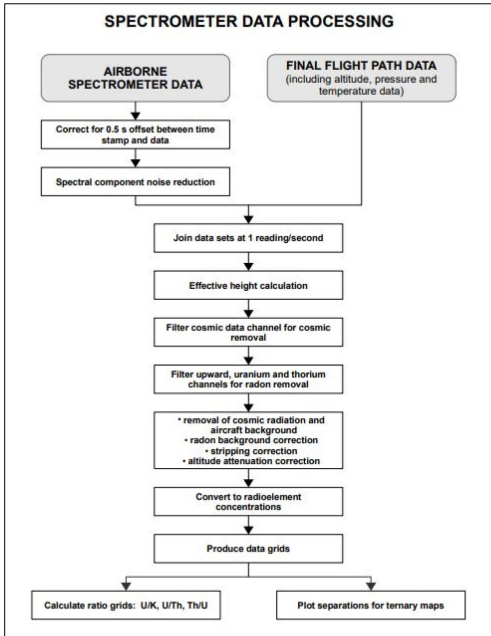
*Figure 30: Spectrometer data processing flow chart*
