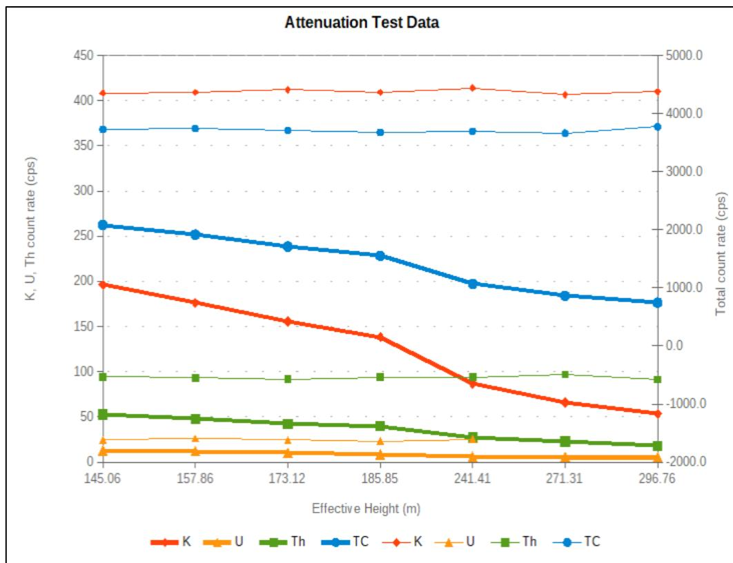
Figure 7: Spectrometer attenuation test: thick lines are recorded data, thin lines are data corrected to an effective height of 60 m using the attenuation coefficients derived.
