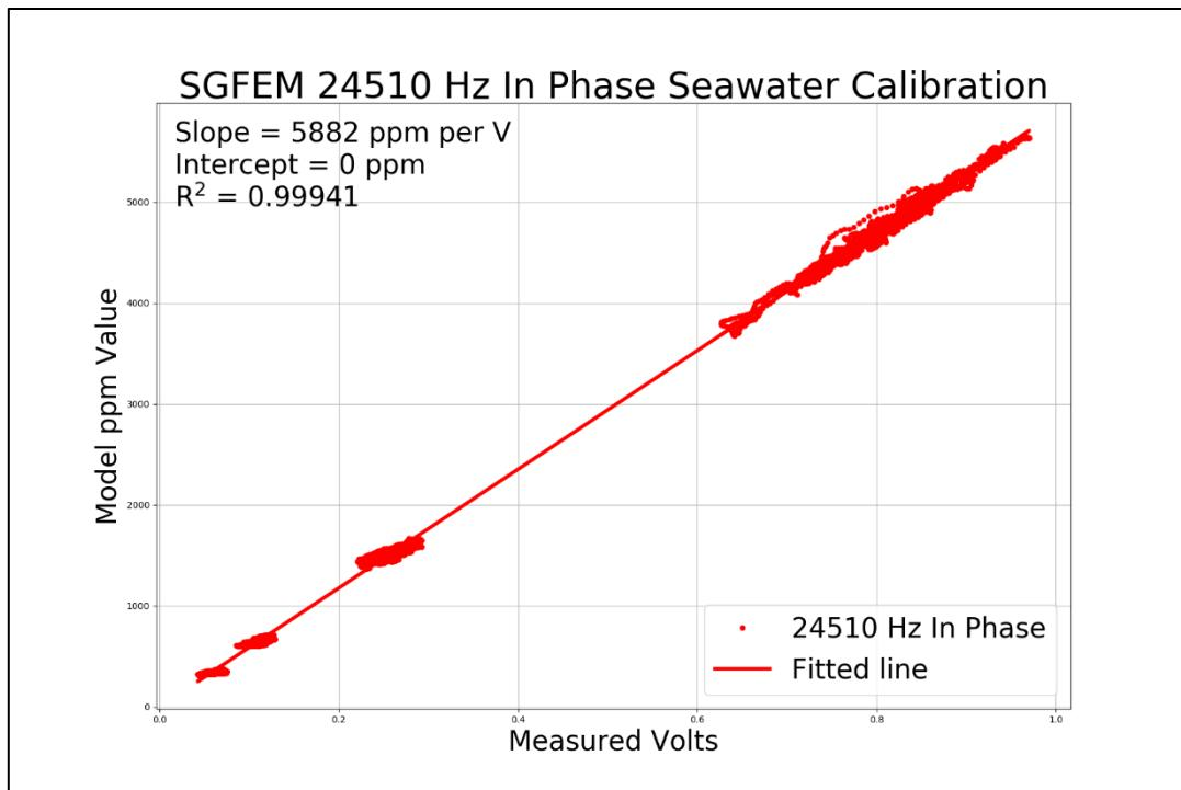
Figure 24: SGFEM 24510 Hz in phase seawater calibration
