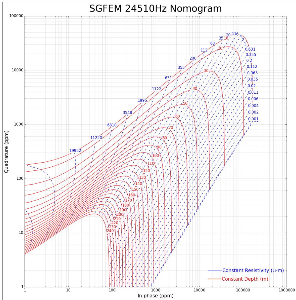
Figure 35: SGFEM 24510Hz Nomogram
