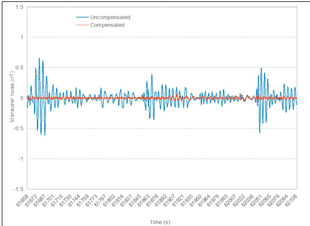
*Figure 6: Tail magnetometer compensation calibration test, June 9, 2020*
