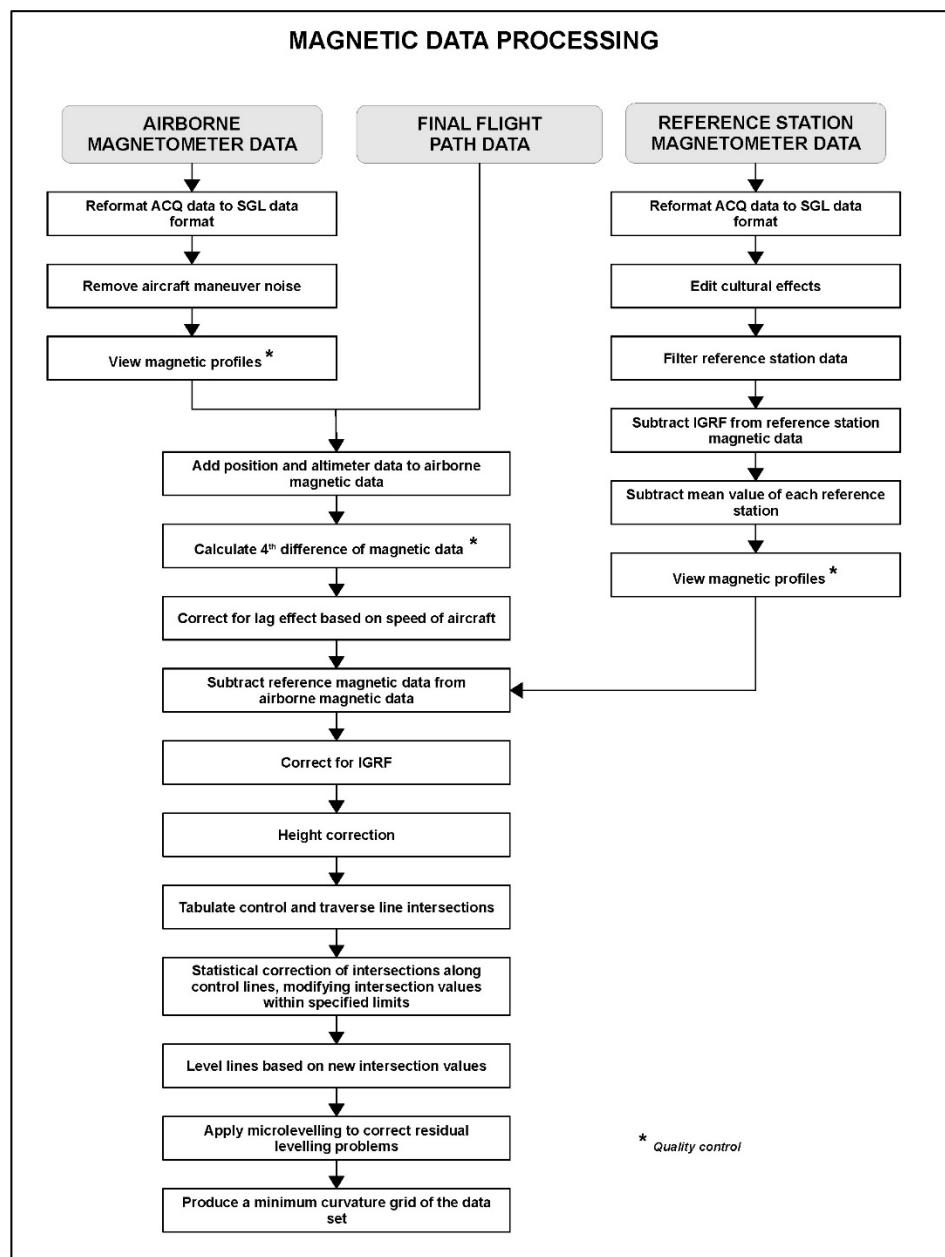
Figure 29: Magnetic data processing flow chart
