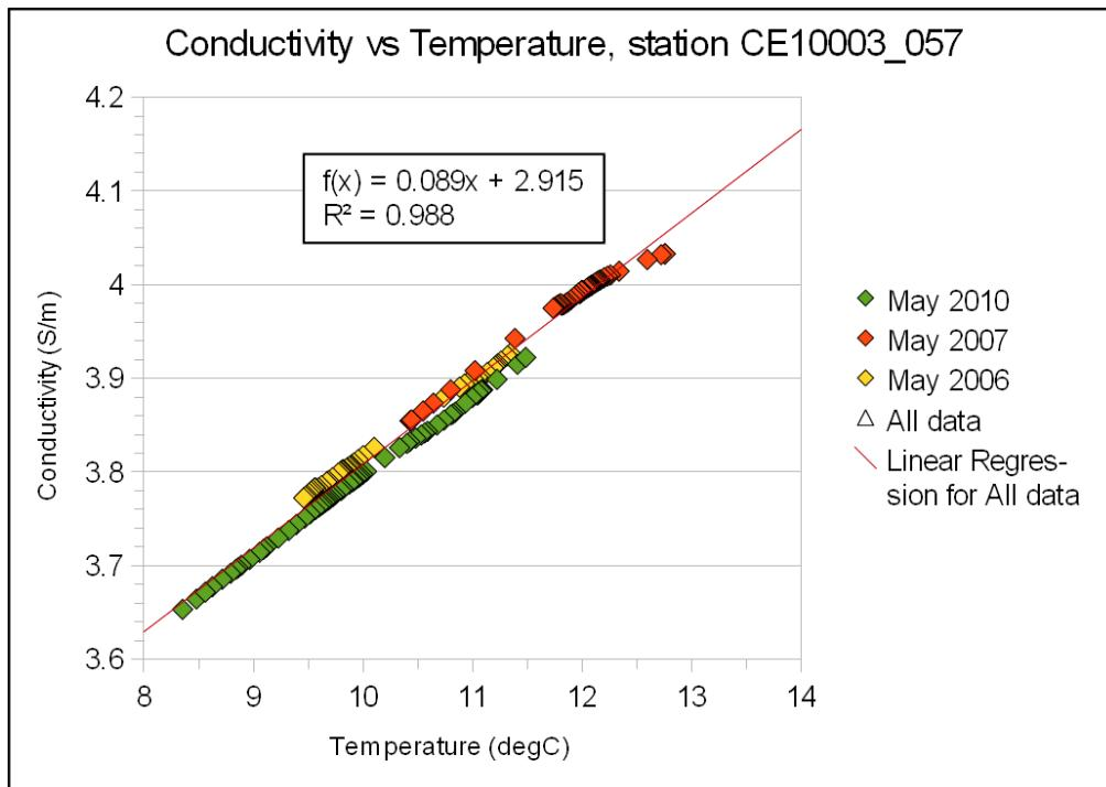
Figure 17: Conductivity variation with temperature
