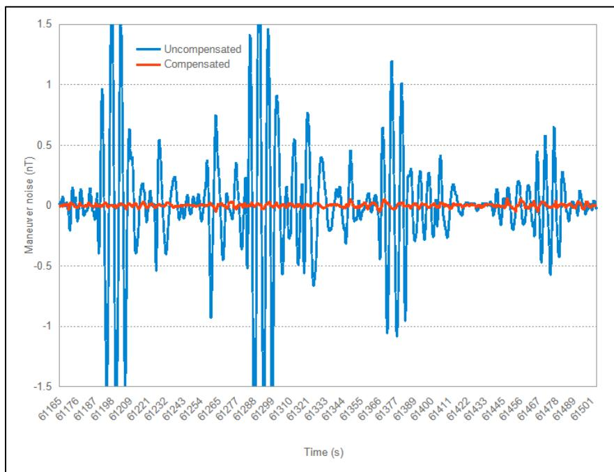
*Figure 8: Tail magnetometer compensation calibration test, May 6, 2021*
