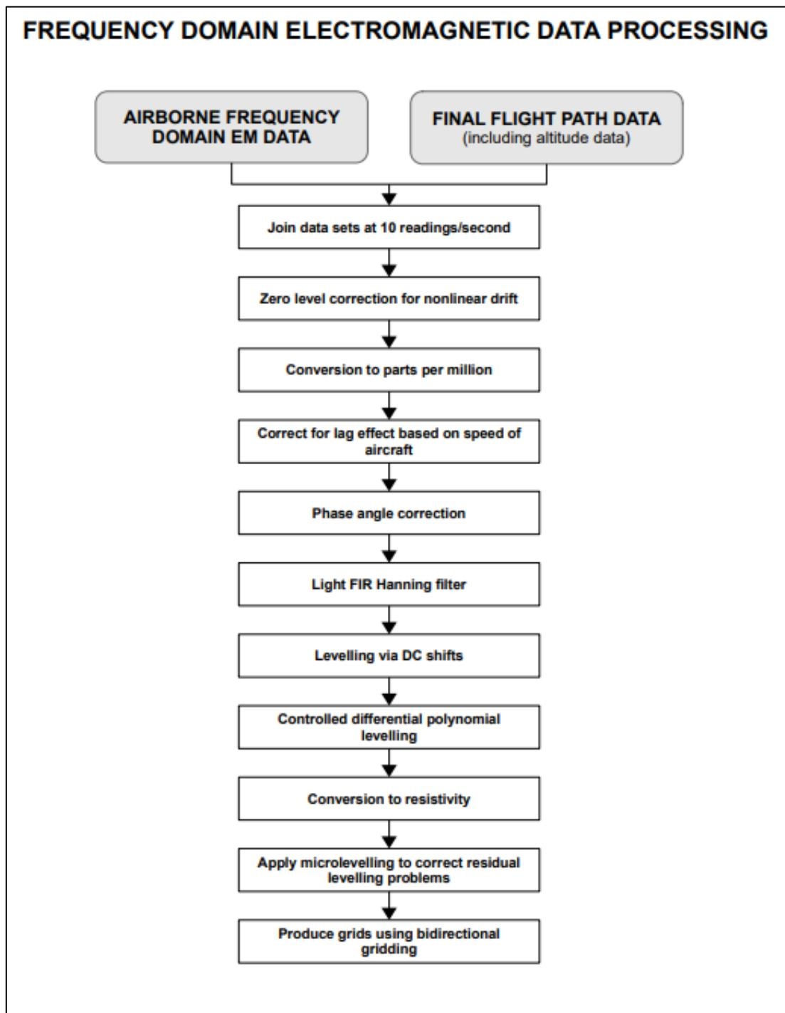
Figure 31: Frequency domain electromagnetic data processing flowchart
