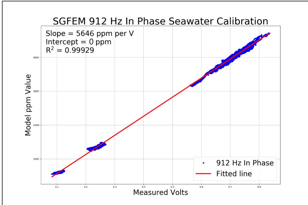
*Figure 21: SGFEM 912 Hz in phase seawater calibration*
