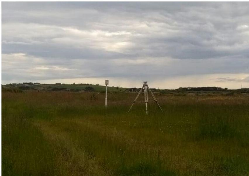
*Figure 27: A standard SGL reference station setup with a magnetometer pole and a tripod mounted GPS antenna*
