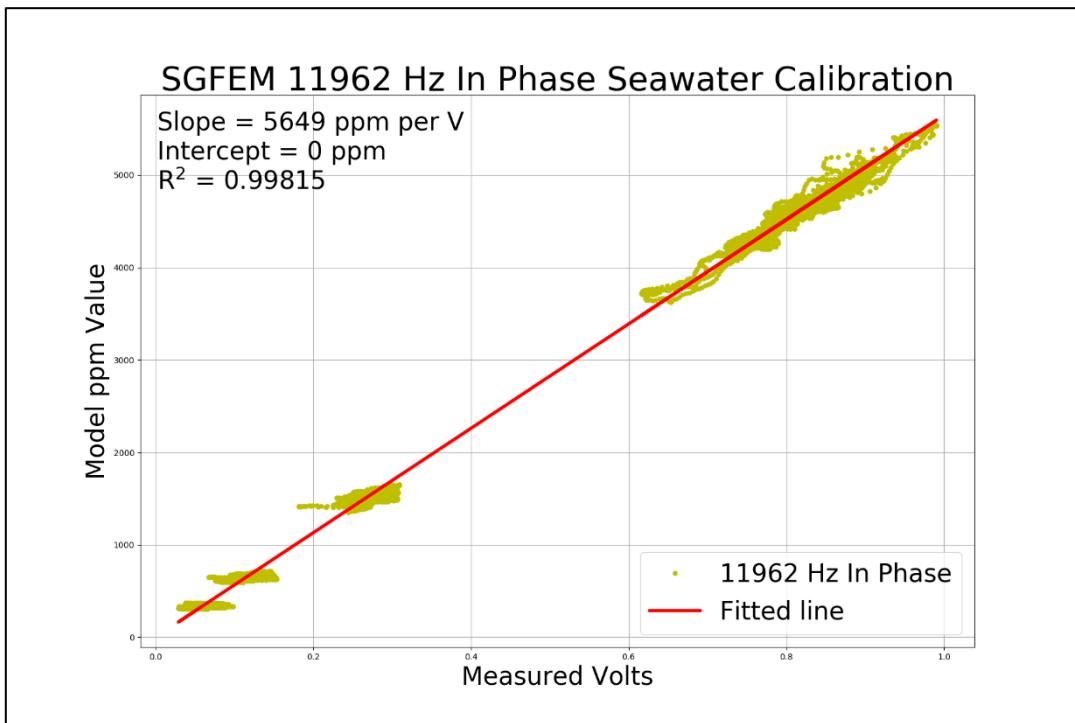
Figure 23: SGFEM 11962 Hz in phase seawater calibration
