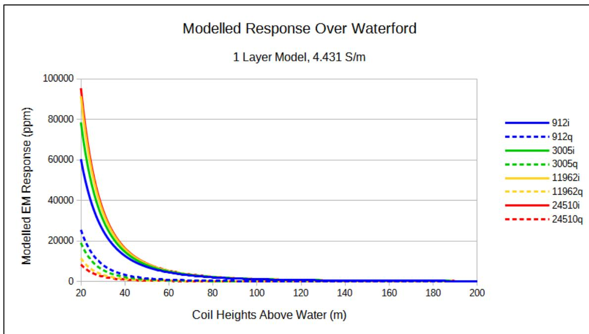
Figure 19: Modelled EM response vs. Coil height above sea water near Waterford
