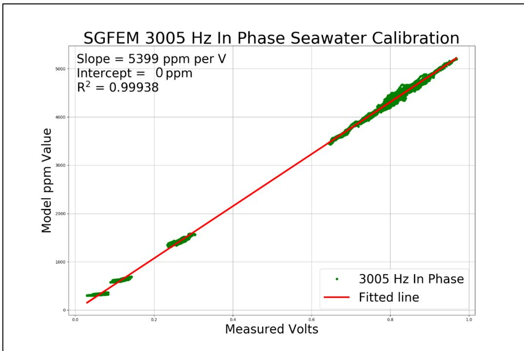
Figure 22: SGFEM 3005 Hz in phase seawater calibration
