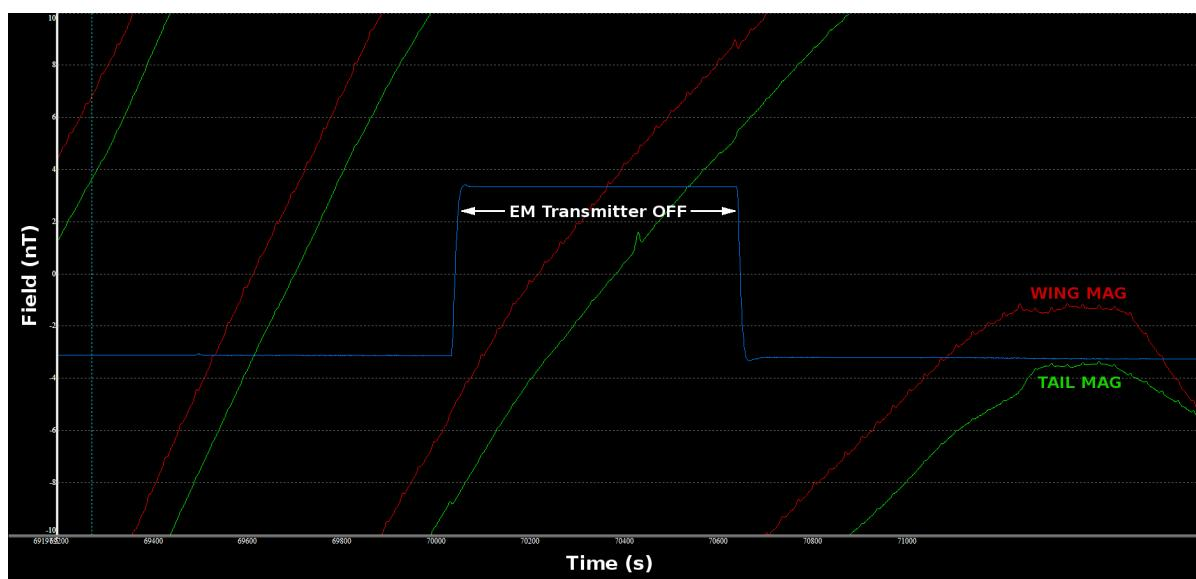
Figure 26: EM transmitter noise test, showing the 4th difference of the tail and wing magnetic sensor traces
