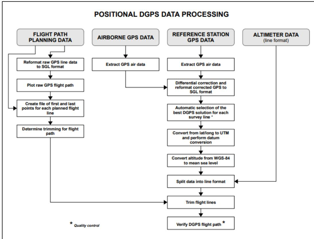
*Figure 36: Positional data processing flow chart*
