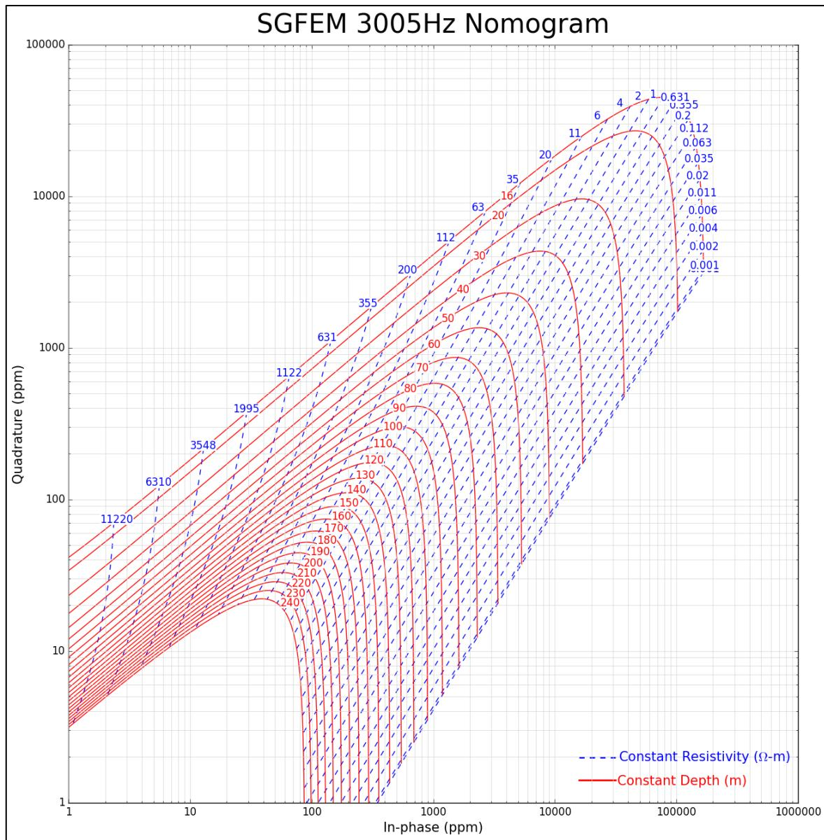
Figure 33: SGFEM 3005Hz Nomogram
