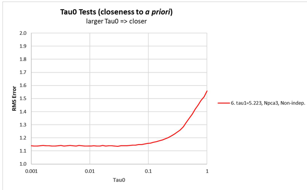
Figure 3.10: \tau_0 versus RMS error curves (L-curves) for a range of different \tau_0 tests (Line L311093, Test Dataset B). Primary details and settings for the tests are annotated in the legend and test numbers correspond with Table 3.1.
