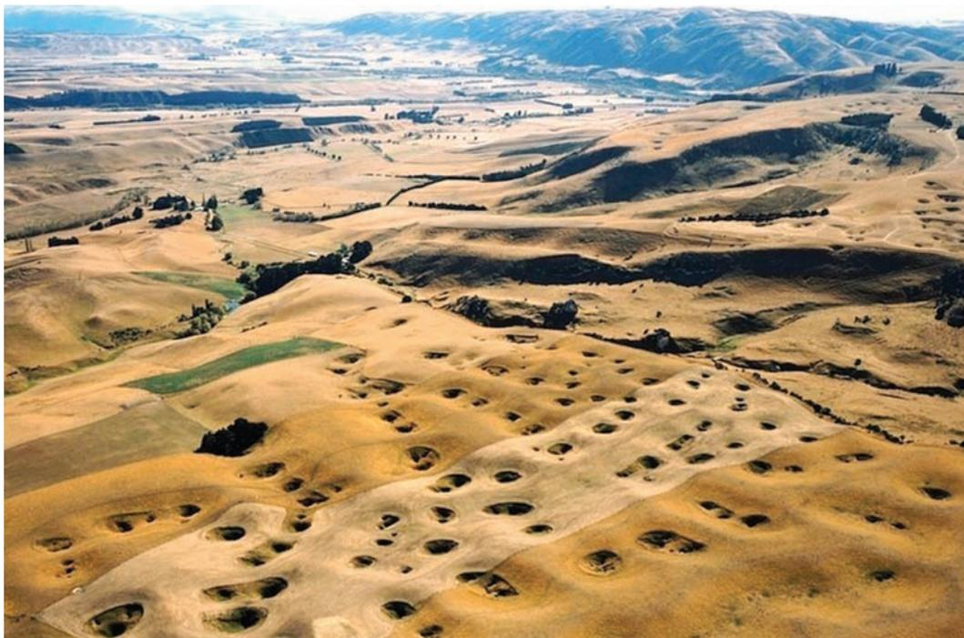
Figure 4.9 Localised recharge to a karst aquifer (New Zealand). In this instance surface landforms (dolines) mark some of these point recharge locations. (Photograph by Lloyd Homer, GNS Science Ltd.)
