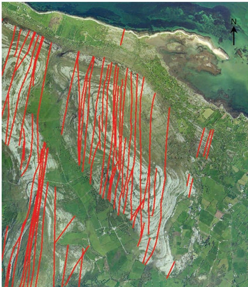
Figure 8.9 Variscan veins oriented almost north-south on Cappanawalla Hill in the northwest Burren. Such veins are major controls on groundwater flow in the Burren (Chapter 7.6). (From Moore and Walsh, 2013b.)
