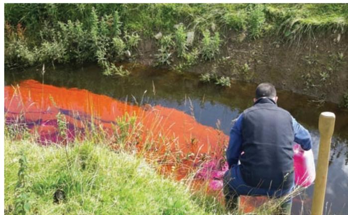
Figure 9.24 Rhodamine dye being injected into a swallow hole in County Roscommon. (Photograph by Caoimhe Hickey.)
