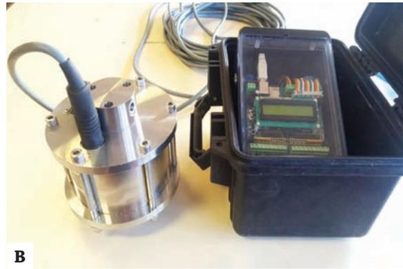
Figure 9.26 (B) A GGUN-FL30 Field Fluorometer and data logger in double waterproof housing. (Photograph by Caoimhe Hickey)
