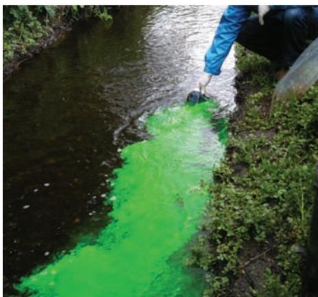
Figure 9.23 Uranine dye being injected in a swallow hole near Ennis (County Clare). (Photograph by Caoimhe Hickey.)
