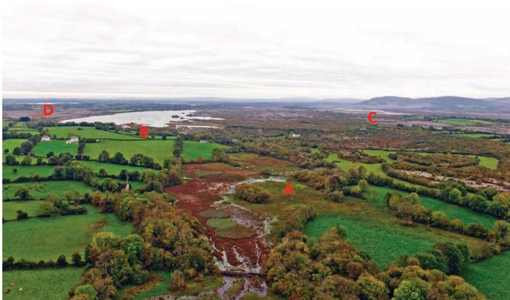
Figure 7.71 The limestone corridor south of Gort, looking south. The Burren plateau is on the right. In the foreground water discharges from a spring (A) which flows north into Galway Bay at Kinvara. The water originates from Lough Bunny (B) which in turn derives its inflow from groundwater originating at the foot of the Burren at Travaun Lough (C). Muckanagh Lough (D) in the far distance drains subterraneously south to the River Fergus. (Photograph by Aerial Eye for David Drew.)
