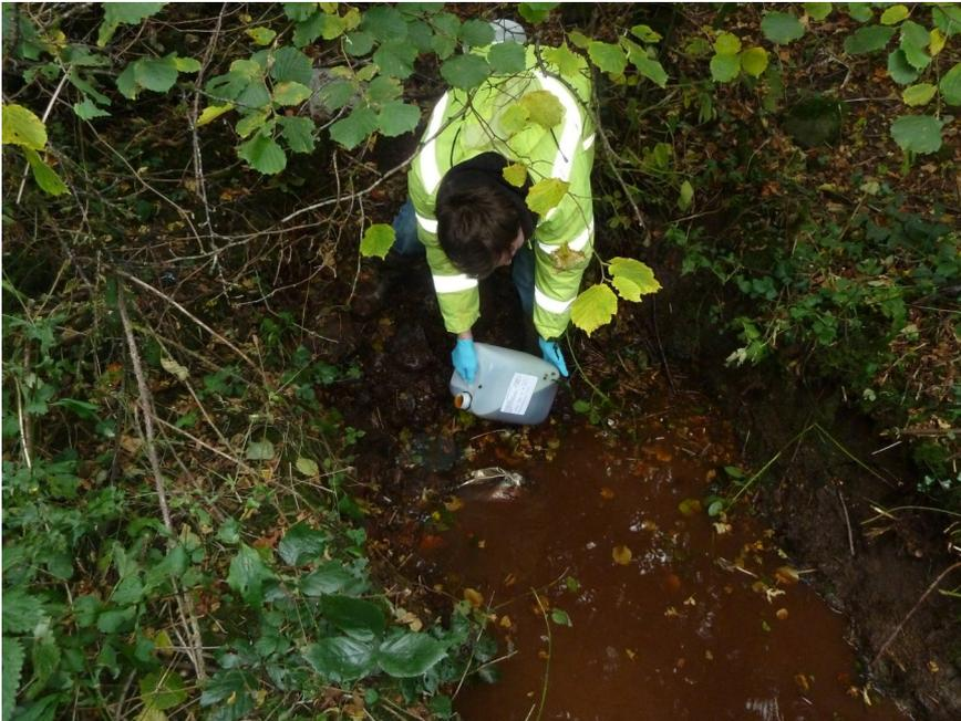
Dye (optical brightener) being injected into swallow hole in wooded area in the above photograph—positively traced to Swinford Spring
