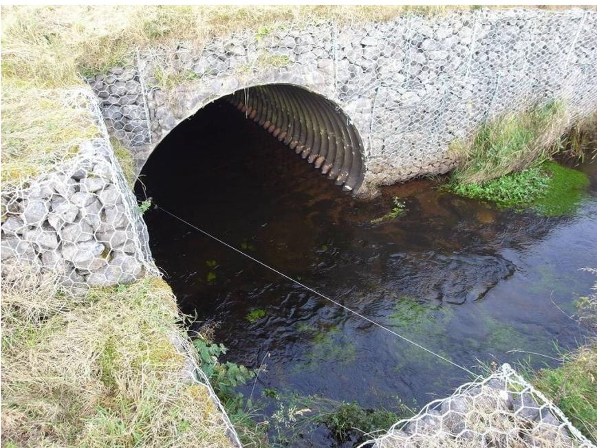
Cotton detector suspended in stream during dye tracer test
