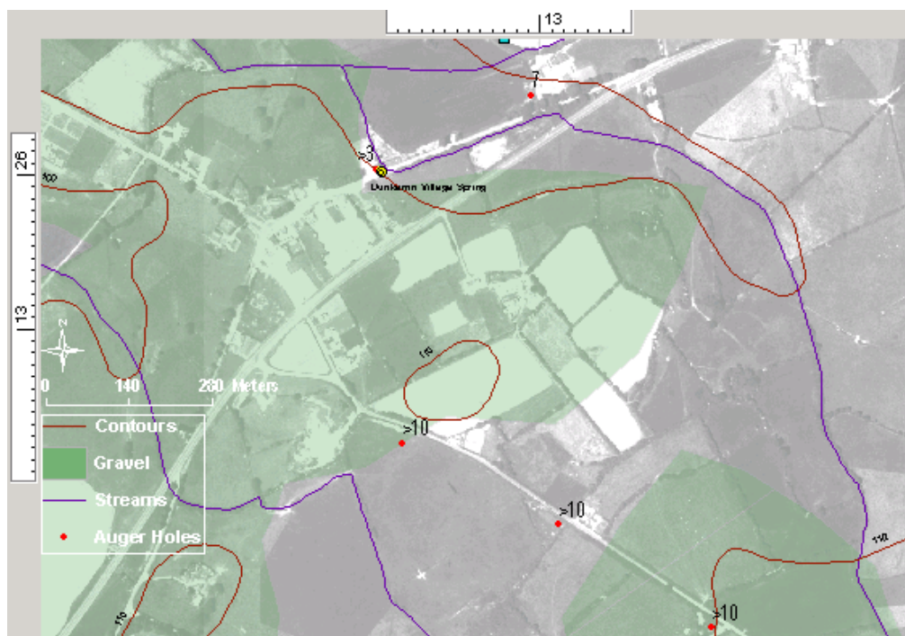
Figure 3 Sand/gravel, contours, streams, location of auger holes and depth to bedrock.
