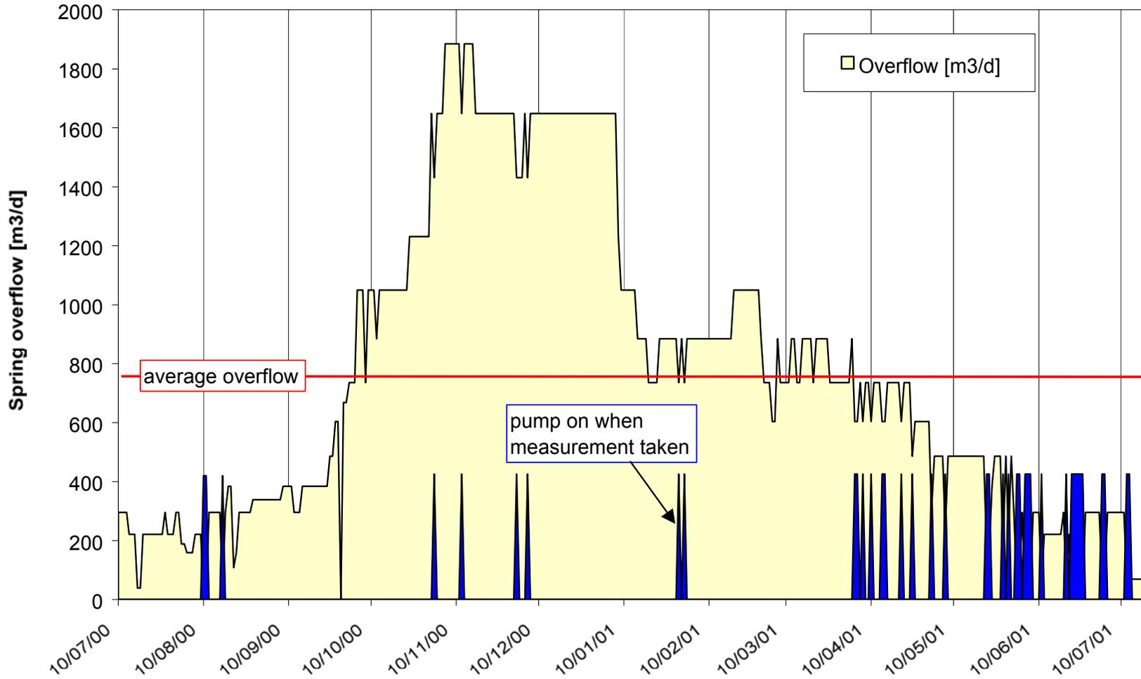
**Figure 4:** Spring overflow, July 2000 to July 2001 (90° V-notch weir).
