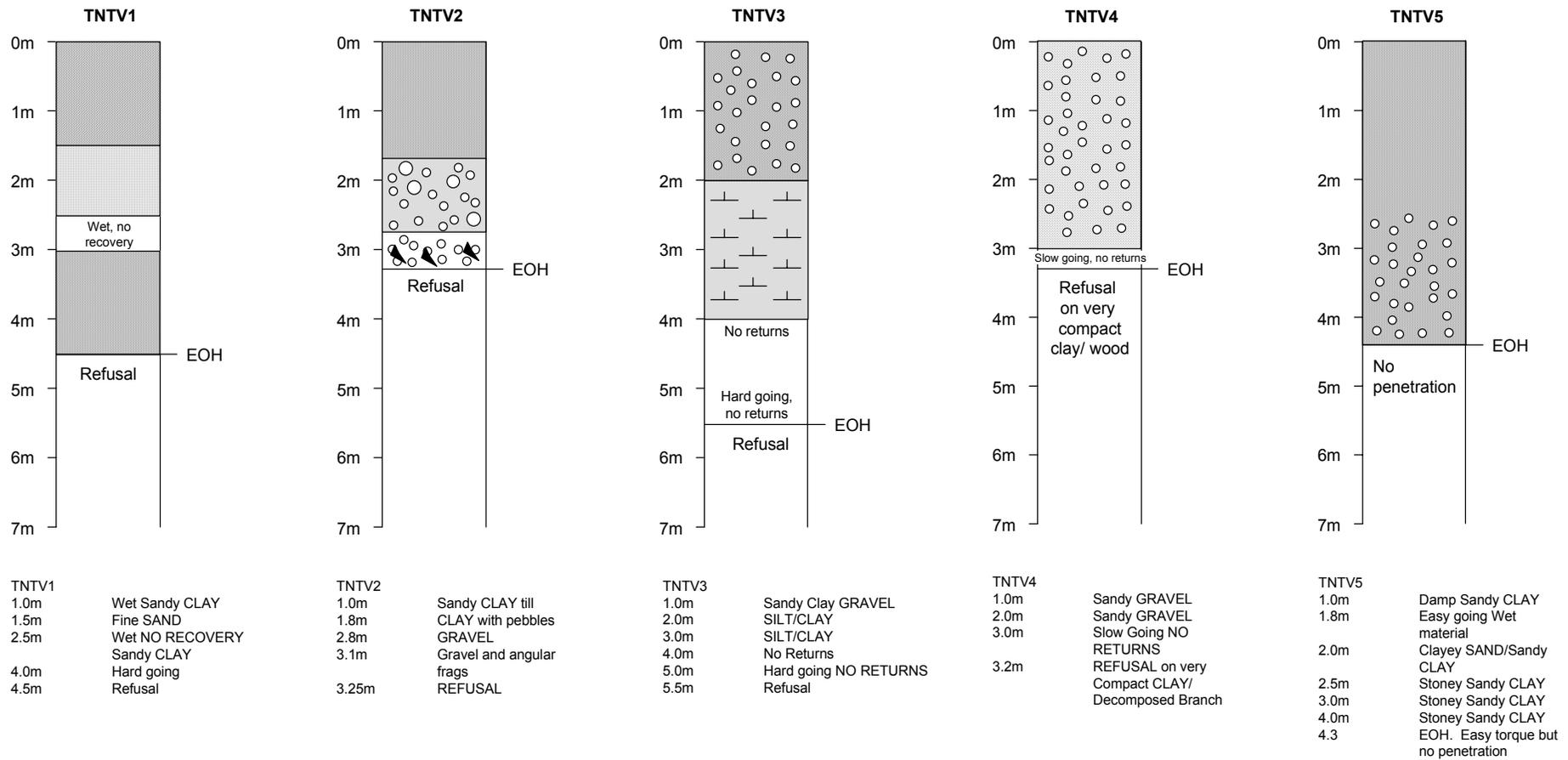
**Figure 3:** Summary logs and lithological descriptions of auger holes drilled to assess depth to bedrock near the Toomyvara spring. (See Figure 2 for locations of the auger holes).
