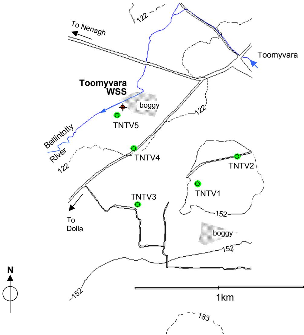
**Figure 2:** Location map of Toomyvara WSS spring. (Showing auger holes drilled by GSI to determine depth to bedrock in the vicinity (TNTV1 to TNTV5) and other hydrogeological features discussed in the text).
