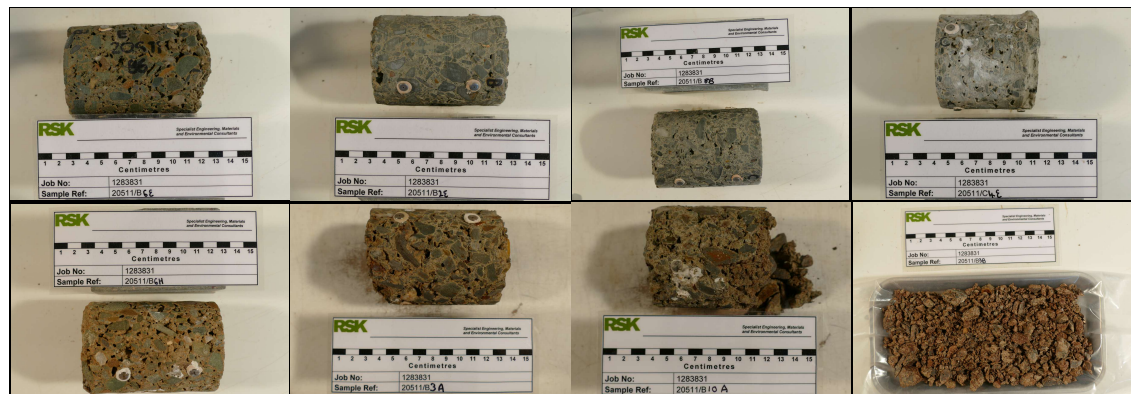
Figure 6-14 Photographs of post-durability test sample condition
