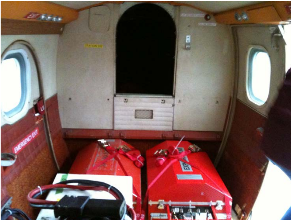
Figure 5: Radiation Solution spectrometer housed in the aircraft.
